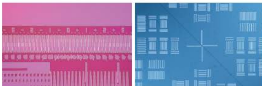
Left Image: Semiconductor (IC wafer) (Objective: TU Plan Fluor BD 50x on Nikon Eclipse microscope)
