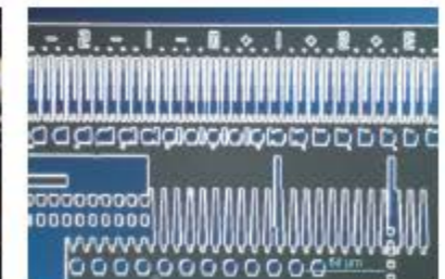
Semiconductor (IC wafer) (Objective: TU Plan Fluor BD 50x on Nikon Eclipse microscope)
